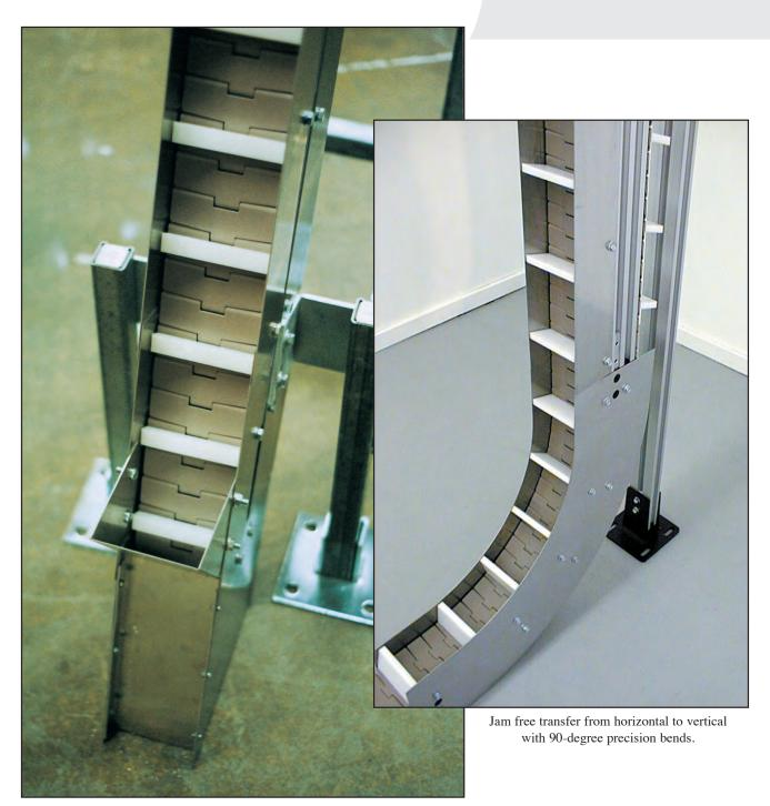
90-degree vertical lift "L" shaped cleated conveyor saves valuable floor space.
